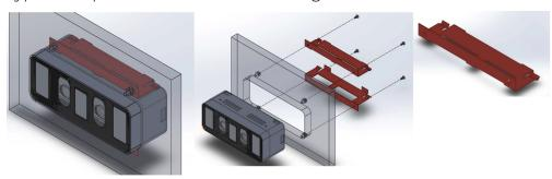
Type B: Side mount using a bracket
