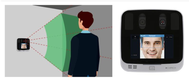
2. Move towards the system to size your face to the LCD display. If the user guide box flashes GREEN, it means you are at an appropriate position. Stop and hold your position until the device captures image of your face and/or iris.
