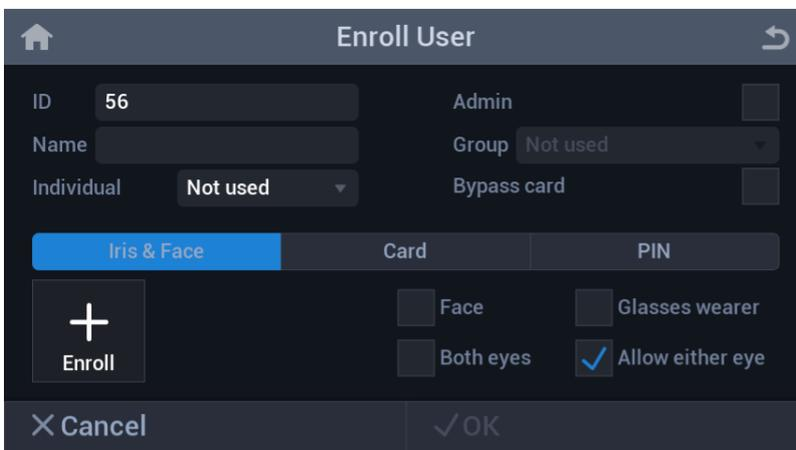
4. Press the plus (+) button in the bottom left to capture image of the new user.
