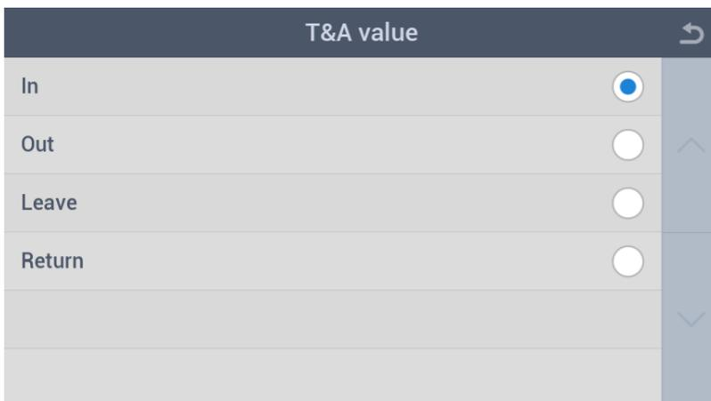
The T&A value menu appears when you select “Fixed (by device)” or “Manual Fix (by key input)” as a T&A mode.
