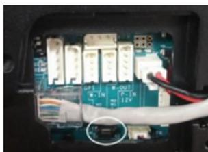
2. Press the button more than 2 secs, which will delete all the data and reset all the settings.
